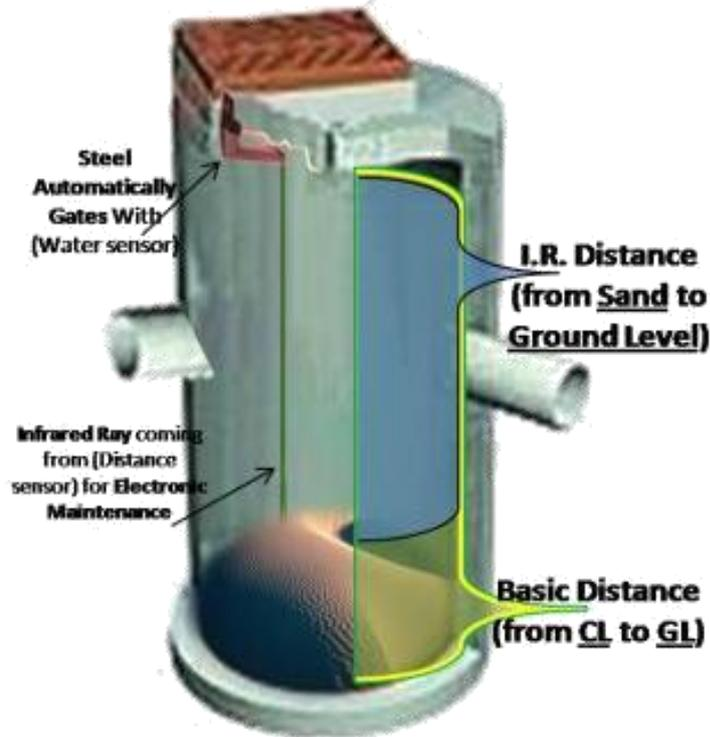
Fig. 7. The Program Equation to calculative sand amount = (I.R. Distance – Basic Distance)
