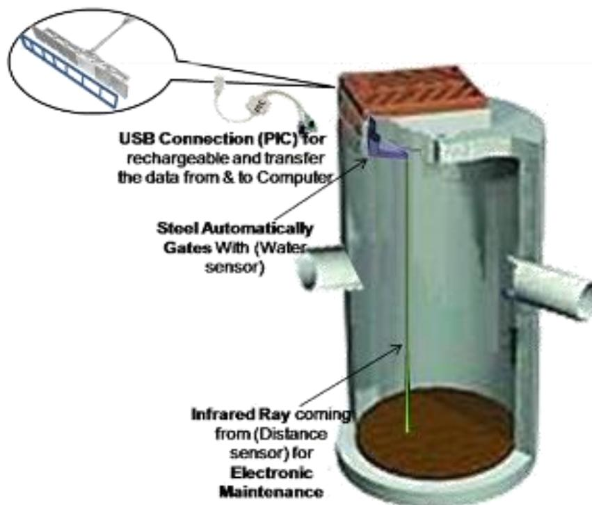
Fig. 1. Device Structure
